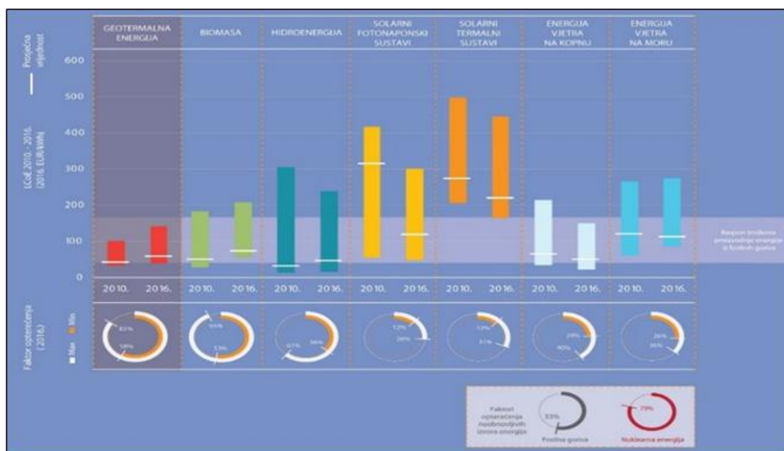
Figure 3: Comparison of capacity factors and LCOE of different renewable energy sources. (Source: Author's adaptation based on the source: Nádor, A. Transitional Danube Region Geothermal Strategy, DARLINGE-Danube Region Leading Geothermal Energy, European Regional Development Fund, 2018.)
