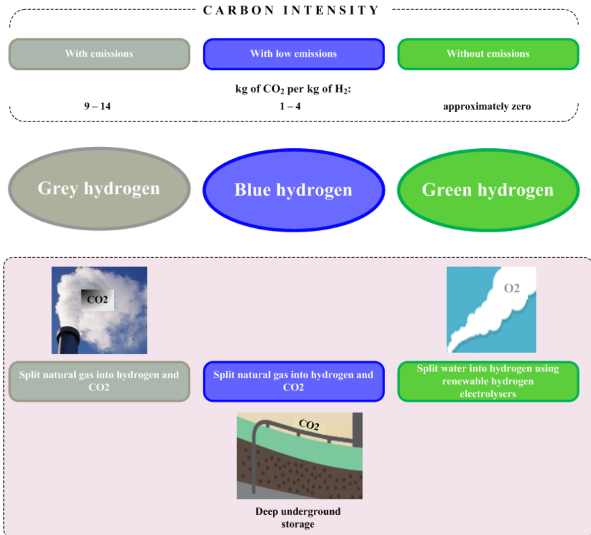
Figure 1: Types of hydrogen marked based on the different methods of its production
